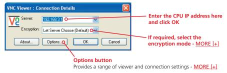
2 In the 'Server:' entry, type the address of the CPU IP as follows:
